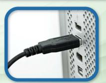
Start by inserting the USB cable into an unused USB port on your computer. No separate power connections are necessary.
